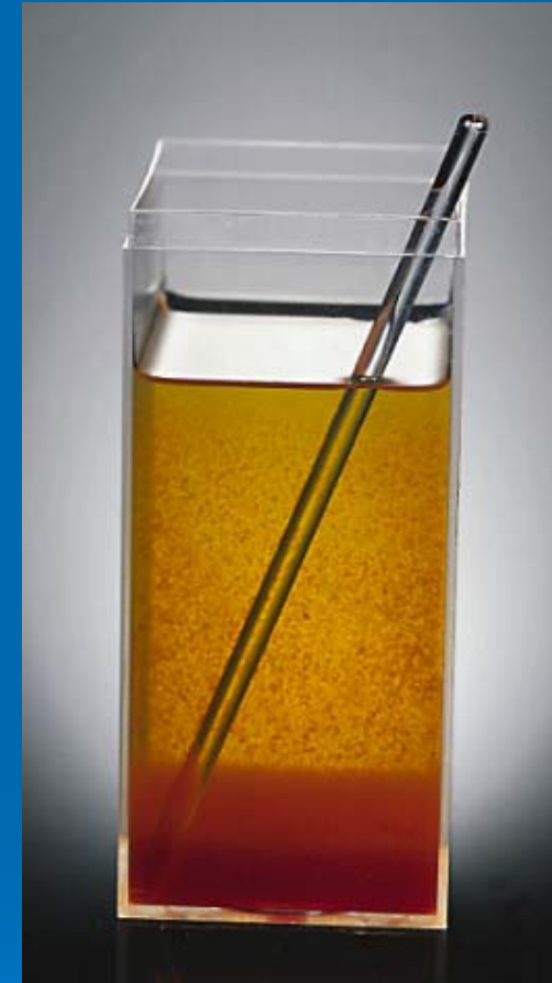
Sol undergoes coagulation upon the addition of Al 2 (SO 4 ) 3 solution
